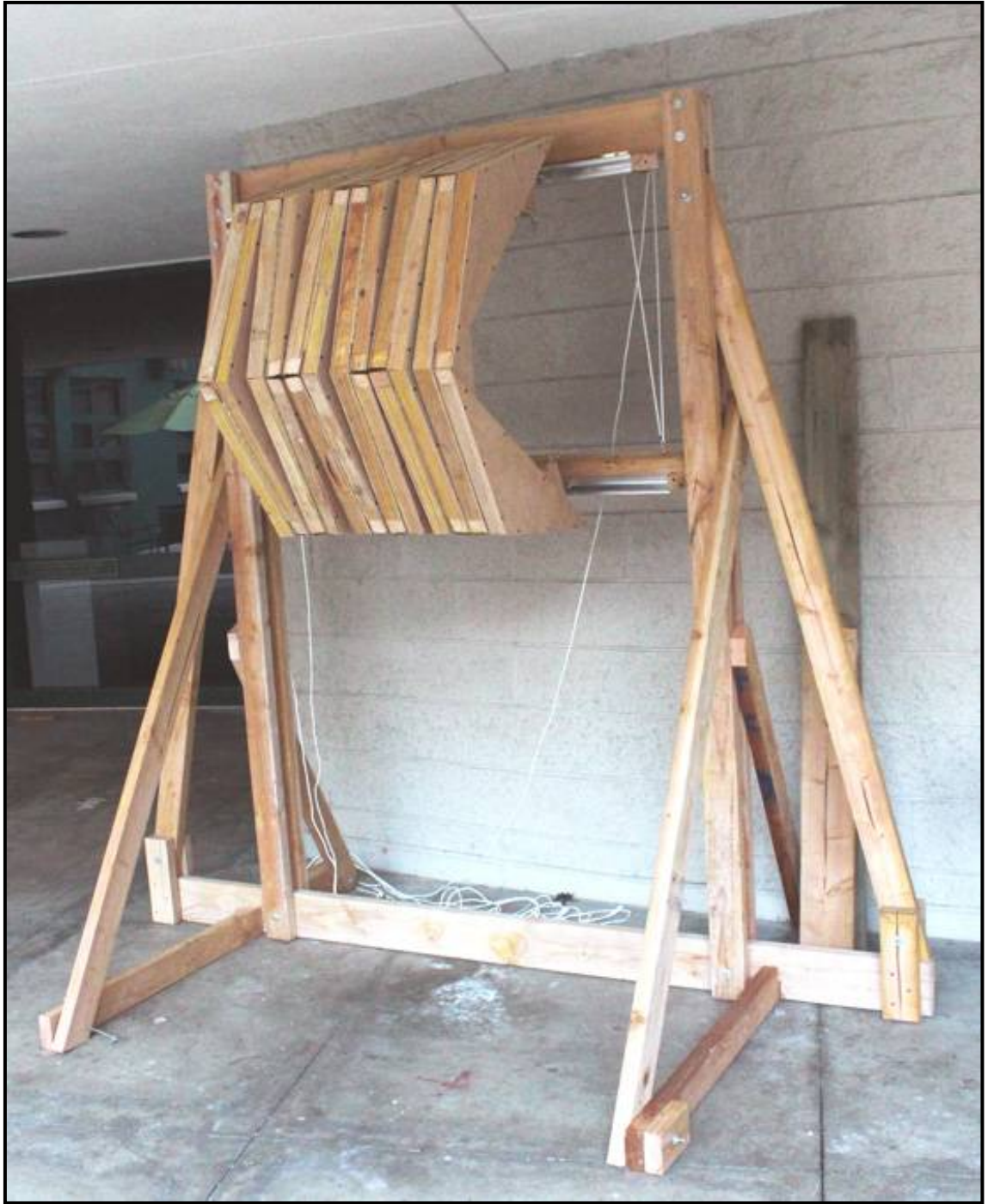
Figure 12.3.4 The large scale prototype in the closed, folded position
