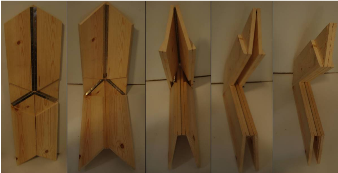
Figure 12.1.1 Small prototype in stages of folding
