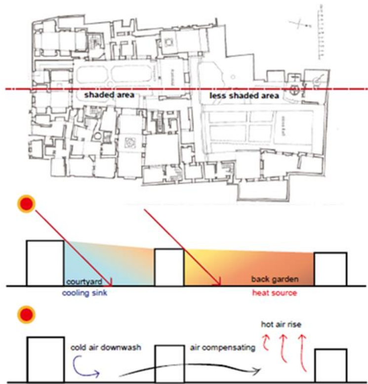
Figure 3-4, why airflow generates and passes through the loggia (drawn by author)
