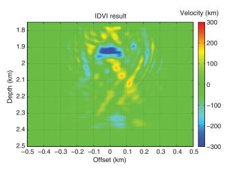
Figure 12. P-wave velocity changes reconstructed using IDWT. A smooth low-velocity zone is resolved within the reservoir. Some scattered velocity changes caused by image noise are also observed.
