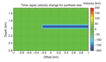
Figure 14. The synthetic P-wave velocity change caused by a fluid injection into a borehole located on the right side of the model.
