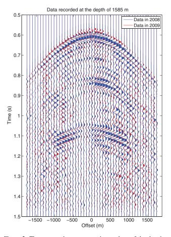
Figure 5. The processed common-receiver gathers of the data in 2008 (blue) and 2009 (red). The receiver is at 1585 m in well 59-2. The data sets are balanced in amplitude and traveltime using their first reflections. The traveltime differences in the later arrivals are the time-lapse-change signals.
