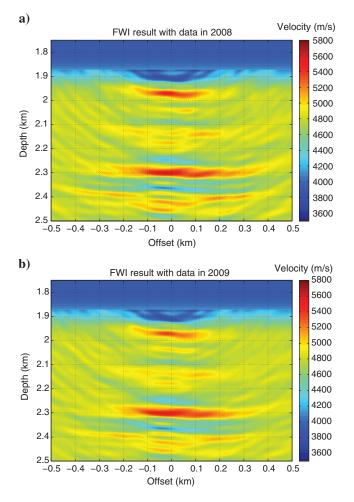
Figure 10. The P-wave velocity model reconstructed using FWI with data from (a) 2008 and (b) 2009. Both models contain similar structures. The 2009 model is shifted slightly downward compared to the 2008 model.
