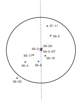
Figure 1. Schematic illustration of walkaway VSP surveys and  $CO_2$  injection and monitoring wells at the SACROC EOR field. The red dots denote the wells with logging records. The green squares denote the two  $CO_2$  injection wells. The blue star marks the VSP monitoring well where downhole receivers are installed. The black circle has a radius of 1 km. The blue dashed line is the walkaway VSP source line.
