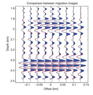
Figure 8. Sample traces from the RTM images of 2008 (blue) and 2009 (red). The lower reflectors in the 2009 image are shifted downward compared to the 2008 image.
