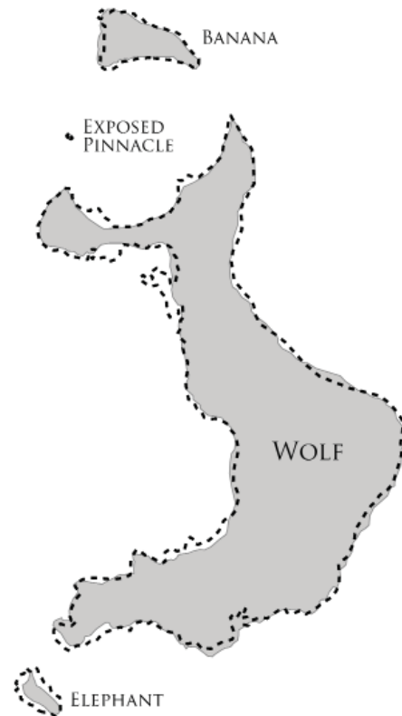
Figure 4. Comparison between the previous mapped coastline (black dashed lines: The Nature Conservancy-CLIRSEN 2006) and the revised coastline determined here (grey areas) of Wolf Island.
