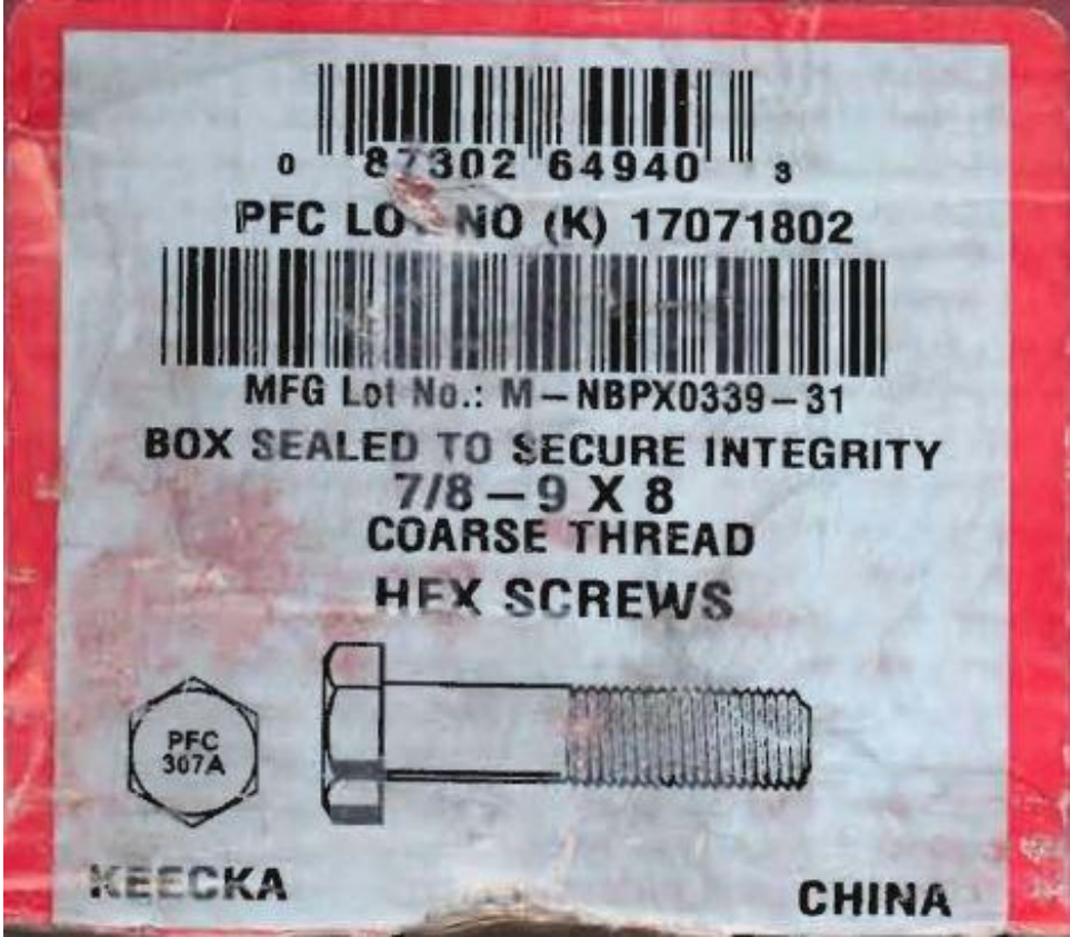
Figure A-21. 7/8-in. (22-mm) Dia. UNC, 8-in. (203-mm) Long Hex Head Bolt and Nut, Test No. MGSMP-1
