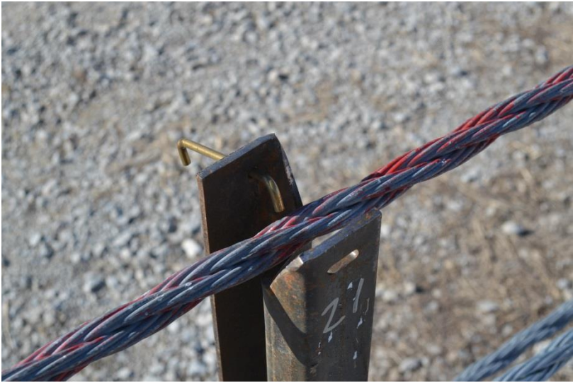
Figure 151. System Damage, Brass Rods, Test No. MWP-7
