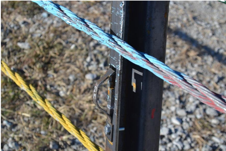
Figure 51. System Damage, Cable Brackets, Test No. MWP-4
