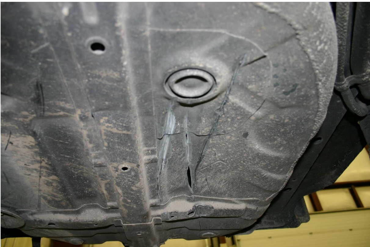
Figure 109. Spare Tire Compartment Penetration, Test No. MWP-6
