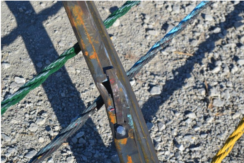
Figure 52. System Damage, Cable Brackets, Test No. MWP-4
