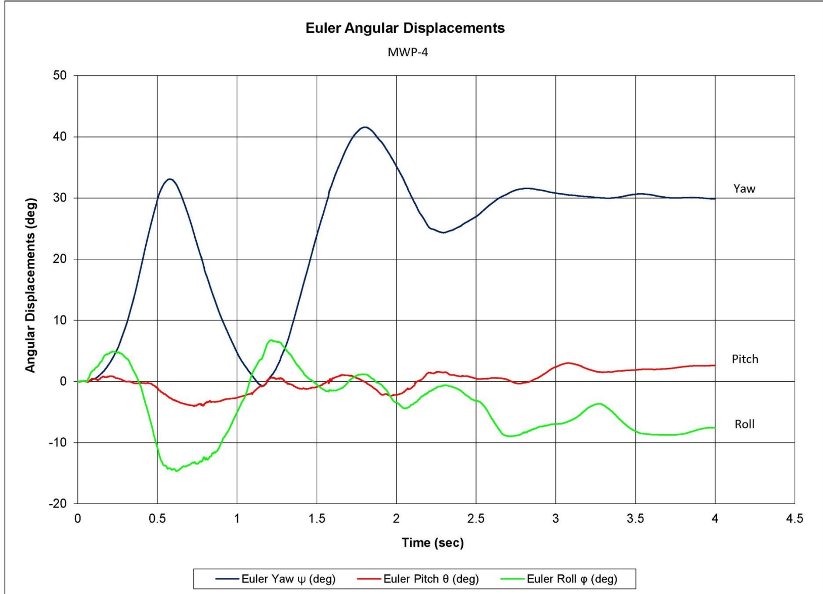
Figure E-7. Vehicle Angular Displacements (SLICE 1), Test No. MWP-4
