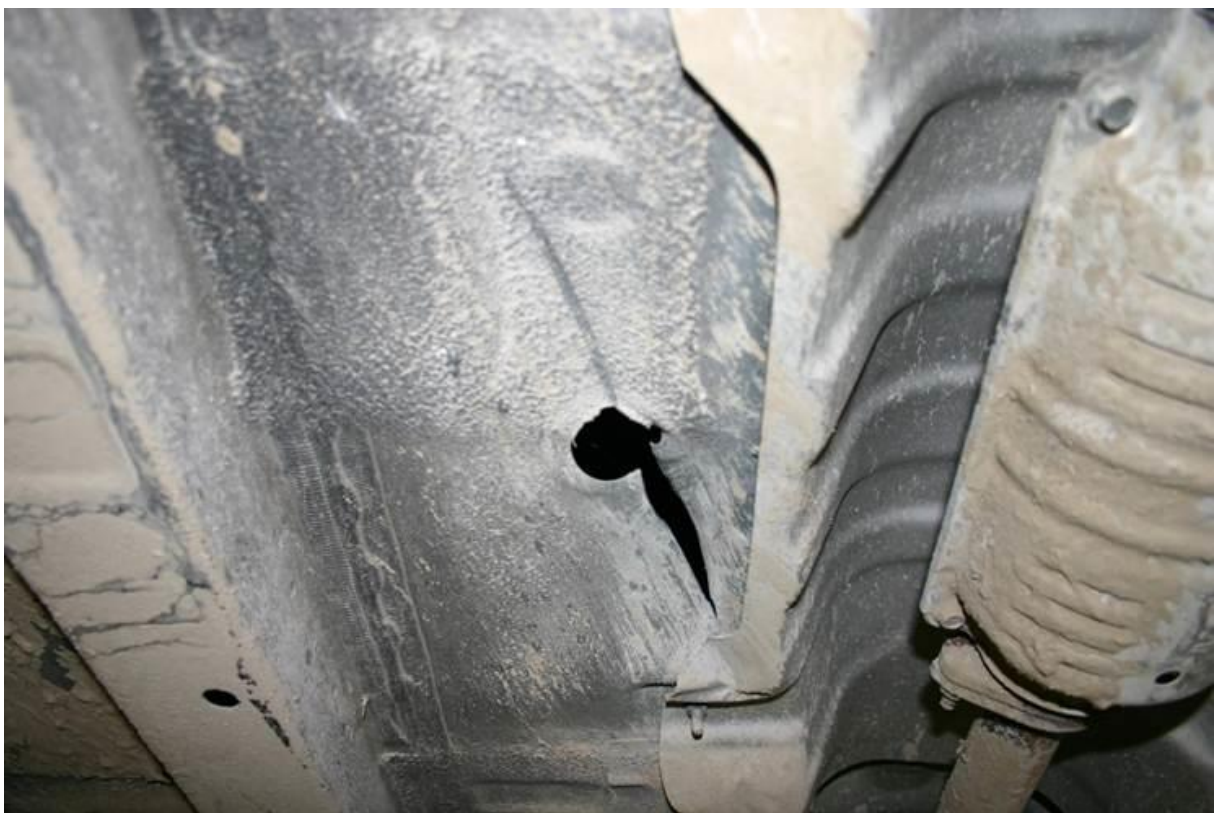
Figure 108. Occupant Compartment Penetration, Test No. MWP-6
