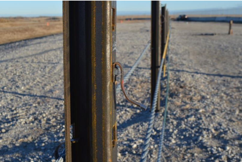
Figure 98. System Damage, Cable Brackets, Test No. MWP-6
