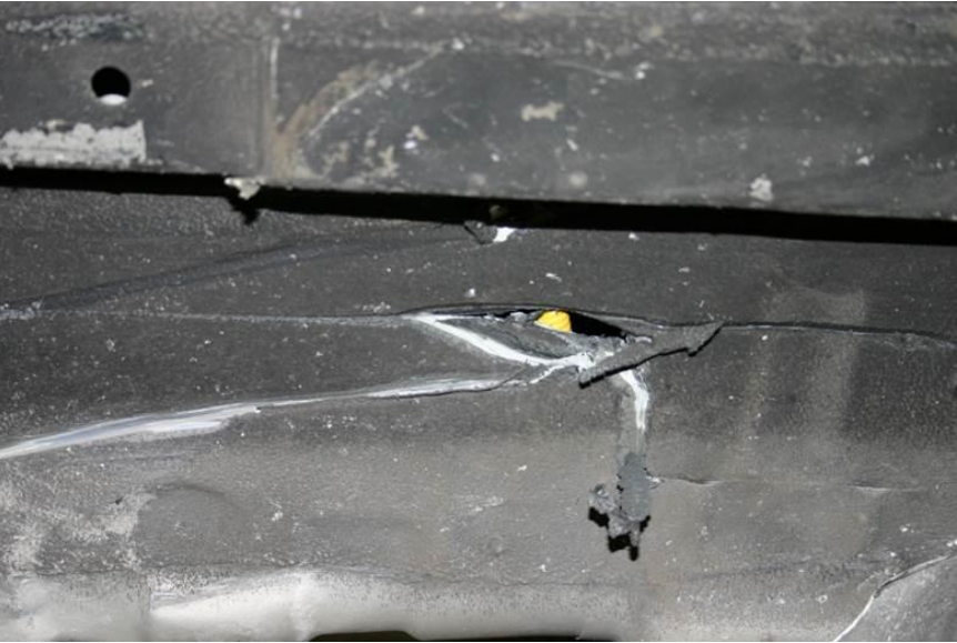
Figure 162. Occupant Compartment Damage, Test No. MWP-7
