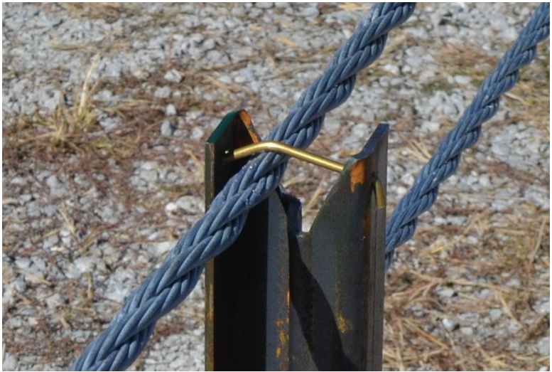
Figure 53. System Damage, Brass Rods, Test No. MWP-4
