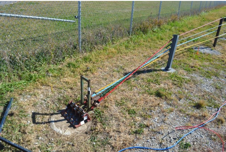
Figure 50. System Damage, End Anchorages, Test No. MWP-4
