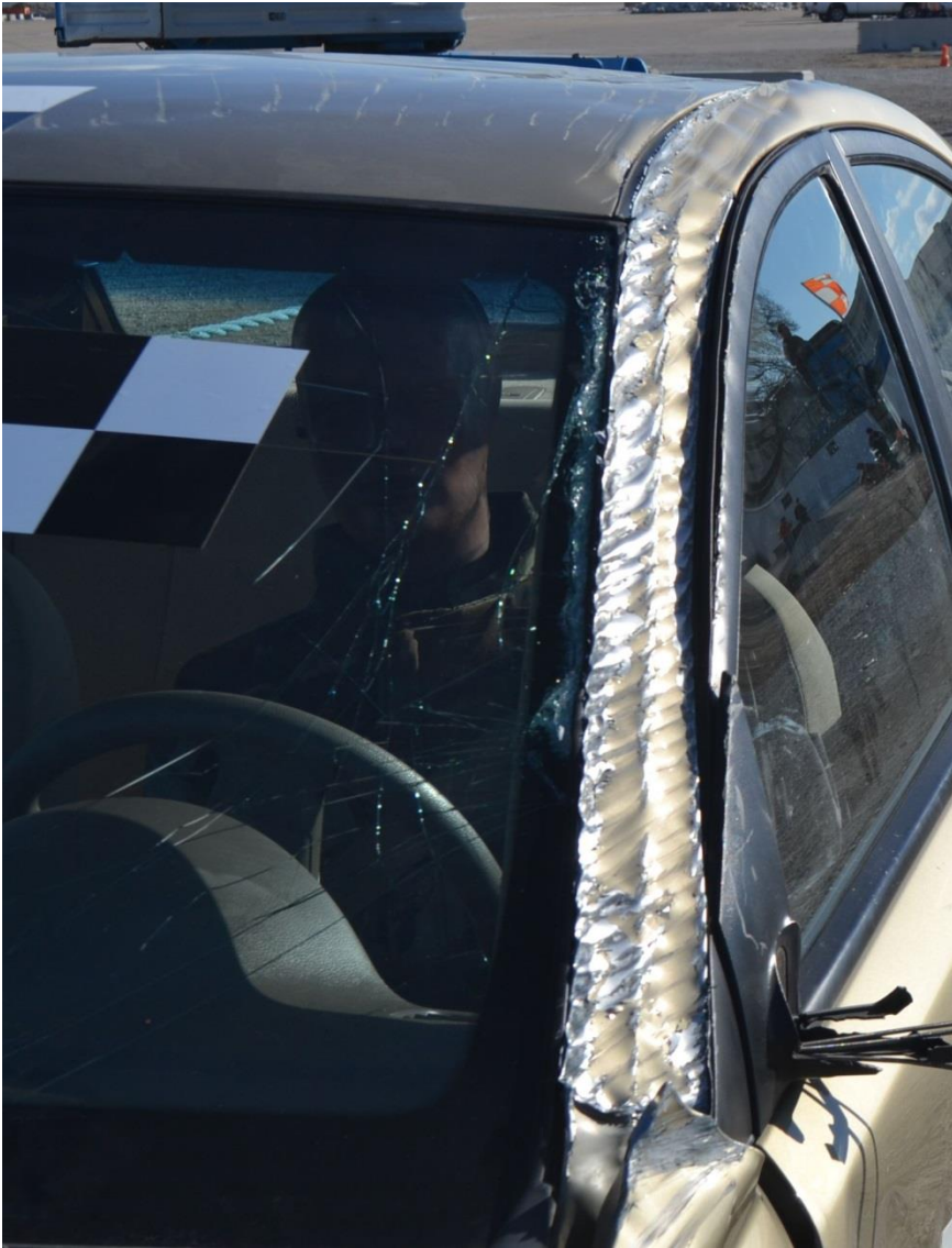
Figure 160. Vehicle Damage, Test No. MWP-7
