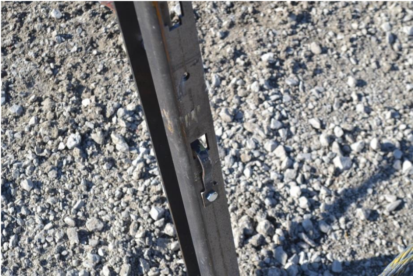
Figure 150. System Damage, Cable Brackets, Test No. MWP-7
