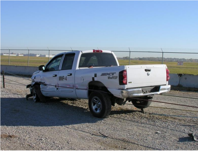
Figure 60. Vehicle Damage, Test No. MWP-4
