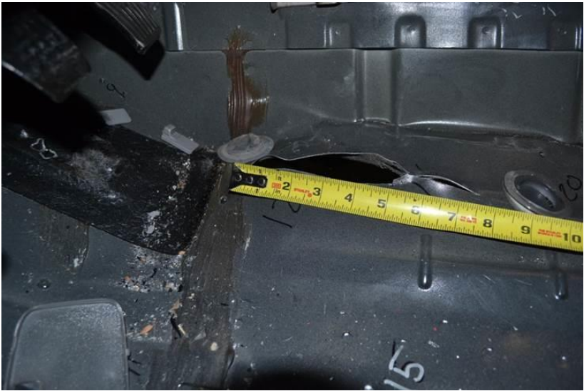
Figure 107. Occupant Compartment Damage, Test No. MWP-6
