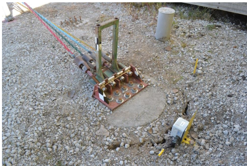
String Potentiometer Test Nos. MWP-4 through MWP-6
