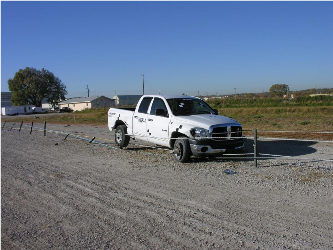
Figure 48. Vehicle Final Position and Trajectory, Test No. MWP-4
