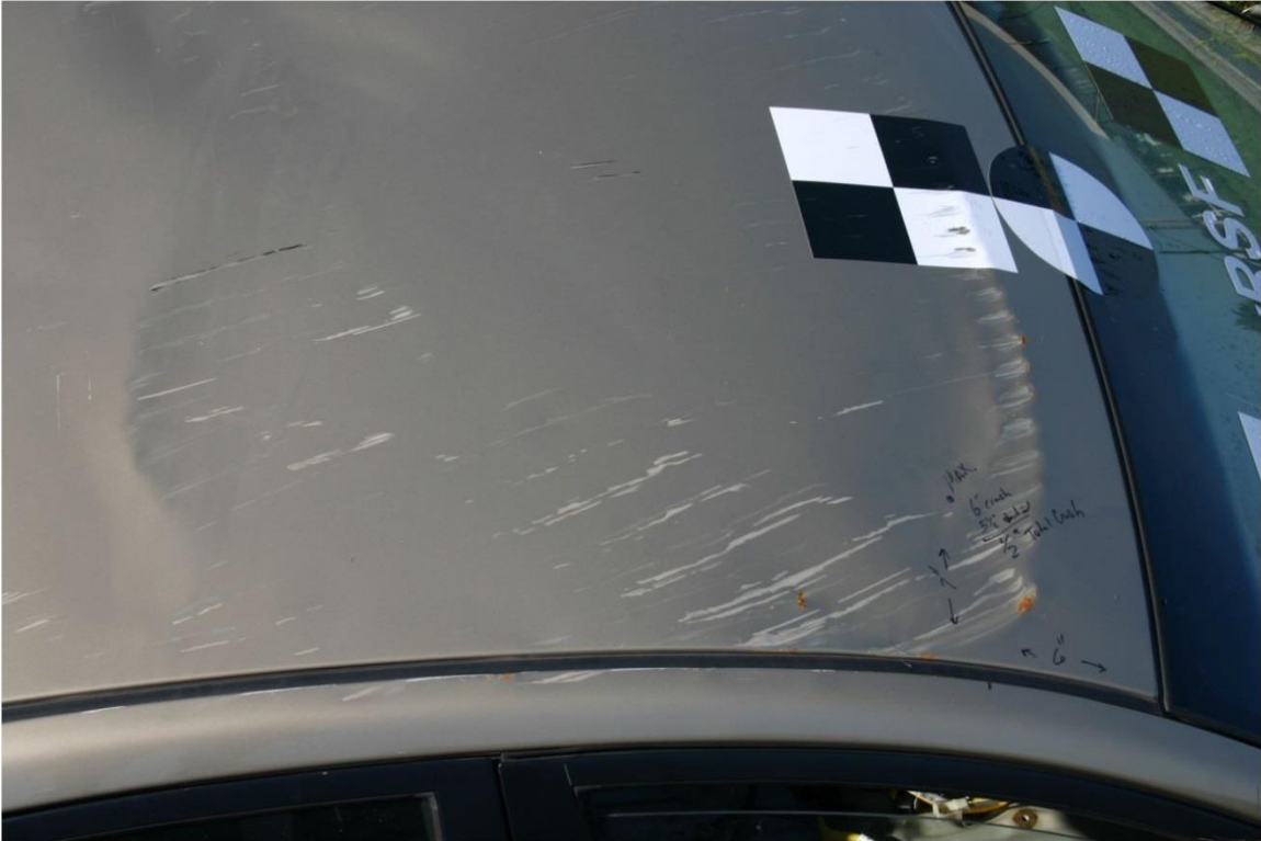
Figure D-18. Roof Deformation Documentation, Test No. MWP-7
