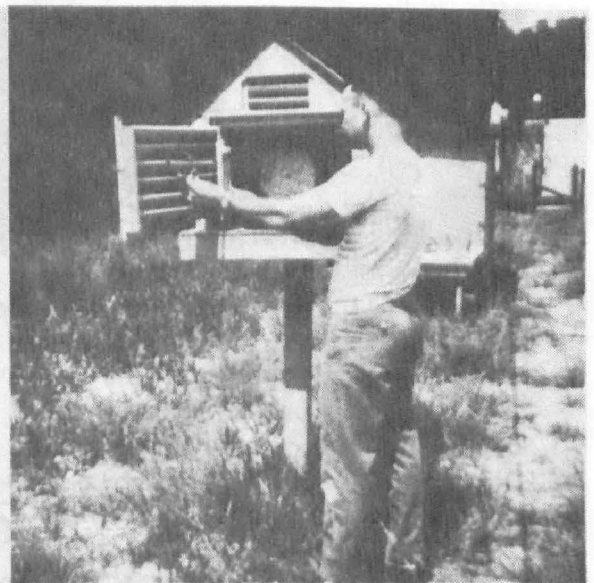
Checking Hygrothermograph at Lake Site
