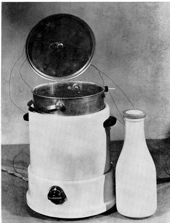
FIGURE 2.—Pasteurizer A, a direct heating, batch-type pasteurizer. There are two thermocouples on the lid and one on the side of the pail at the left. Size of the appliance may be compared with that of the quart bottle of milk.
