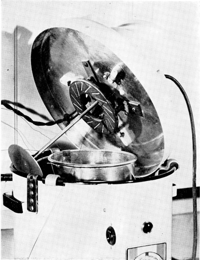
FIGURE 5.—Pasteurizer B equipped with a lid heater. The agitator is also shown.
