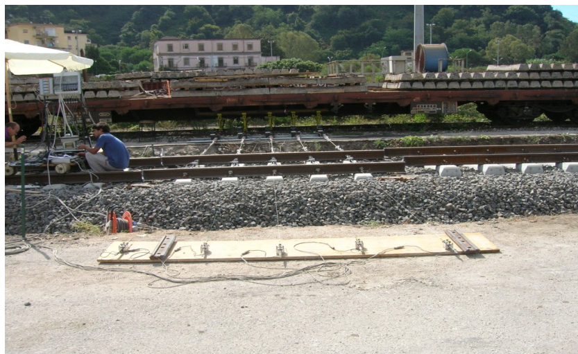
Figure 6: Alternative DCPPT layout for lateral resistance evaluation.
