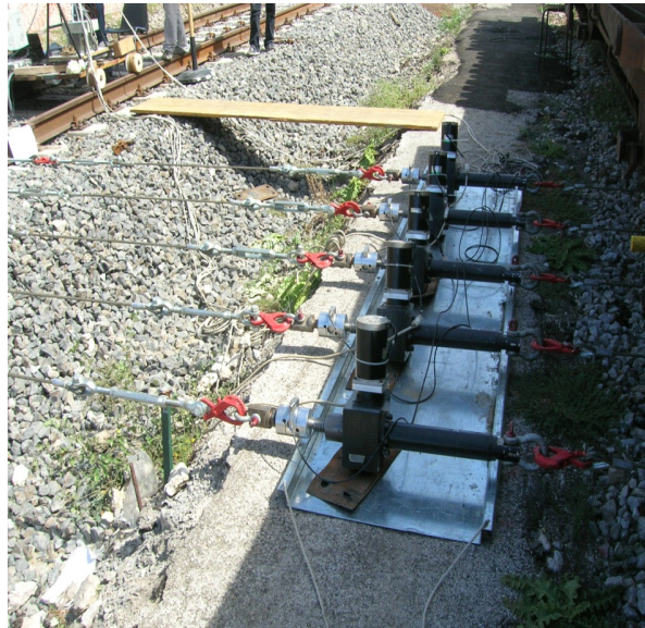
Figure 7: Electromechanical actuators in pulling position.
