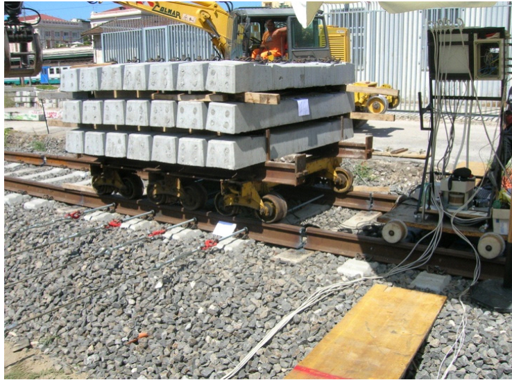
Figure 12: DCPPT in the loaded-track configuration.
