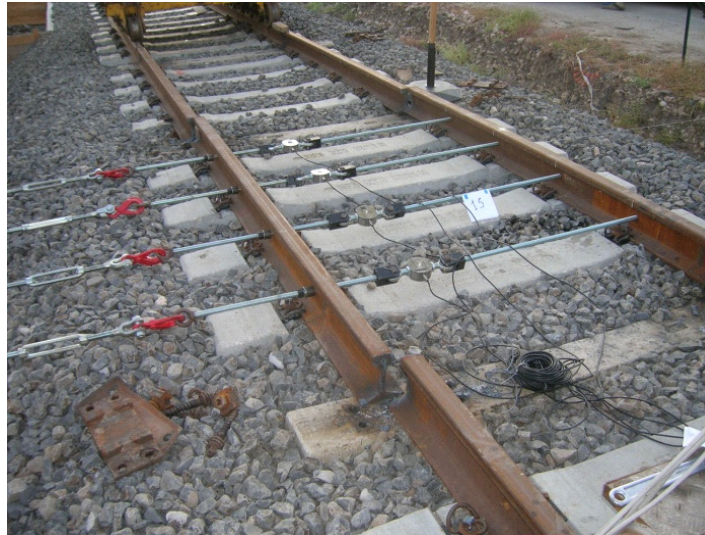
Figure 9: Actuators connection to the rails.
