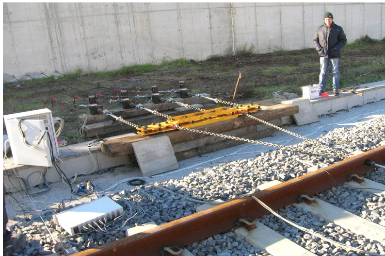
Figure 11: Test setup adopted for the transverse test of the continuous track.
