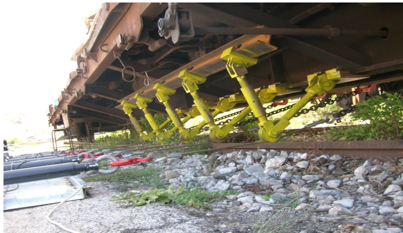
Figure 8: Actuators connection to the beam of the contrast wagon.
