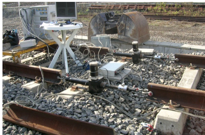
Figure 5b: Physical testing set-up adopting DCPPT layout.
