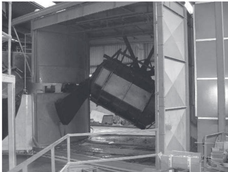
Figure 1.5 Rotationally moulded skin-foam boat hull is being made inside the mould in a single manufacturing step (Crawford, R. J. K., M.P, 2003).
