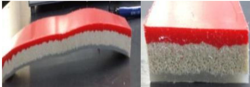
Figure 1.3 Rotatorially moulded skin-foam-skin three layer sandwich structure.
