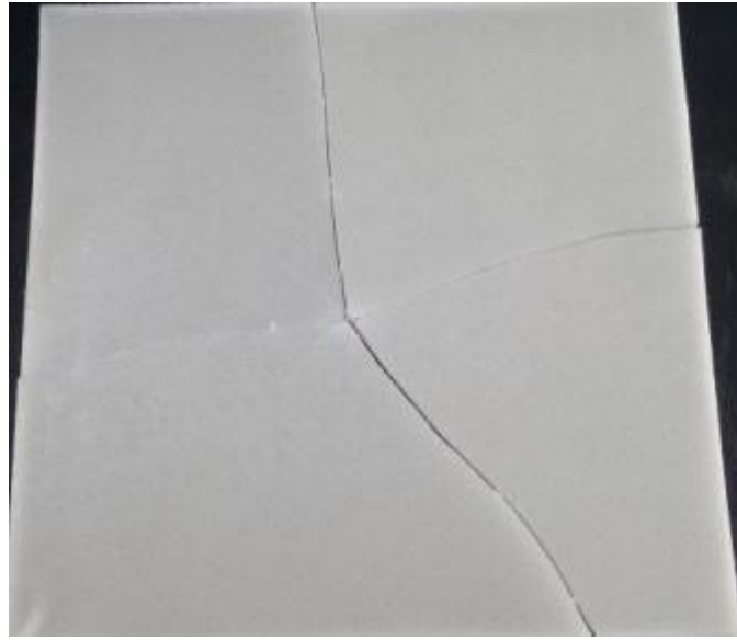
Figure 5.10 Typical brittle failure of PP samples.
