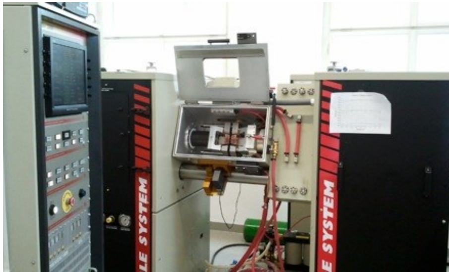
Figure 3-17 - Gleeble dynamic material research system
