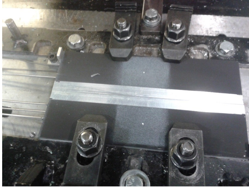
Figure 5-66 – Pre-weld setup for DIC showing painted work pieces, thermocouples and support structure
