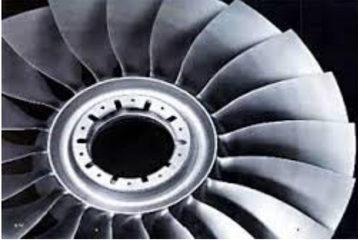
Figure 2-2 – Turbine assembled by linear friction welding [4]
