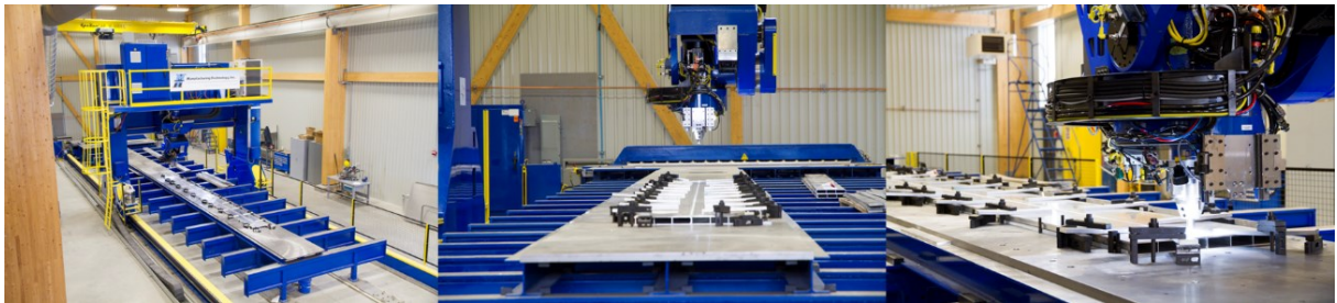
Figure 5-23 – CEE-UQAC FSW machine
