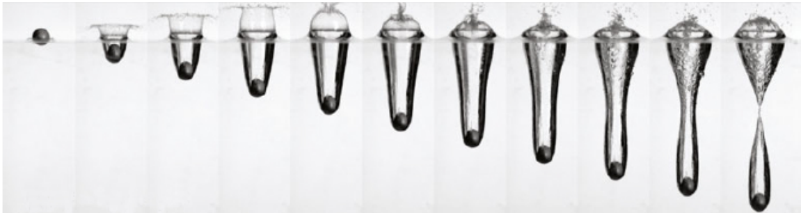
Fig. 1.1: The water entry of a steel sphere [6] showing the different phases from impact to pinch-off.
