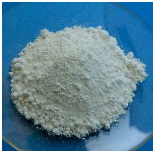
Figure 5.7: \text{CeO}_2 in powder form before sintering [45].
