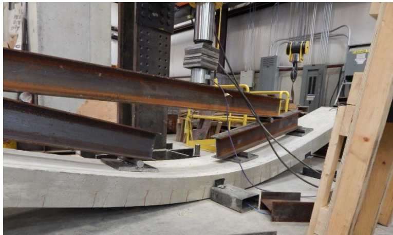
Figure 5 – Maximum deflection of SR3, note the well distributed cracking
