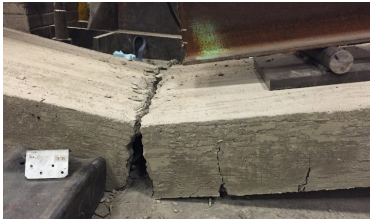
Figure 7 – SW14 Ruptured Wire Failure
