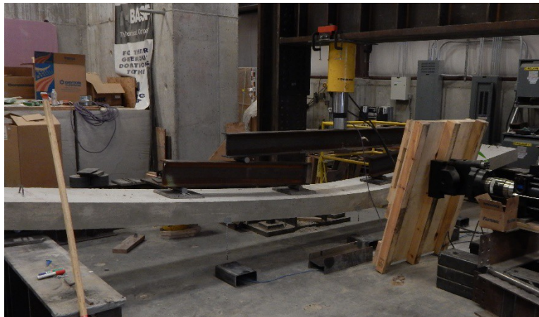
Figure 5 – Maximum deflection of SR3, note the well distributed cracking
