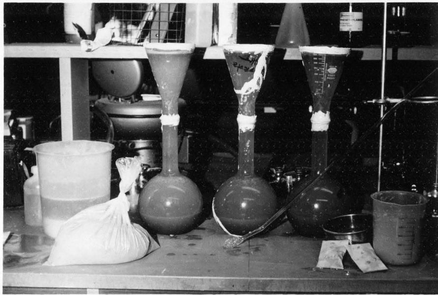
Figure 19. Apparatus employed for the separation of roots from the soil.
