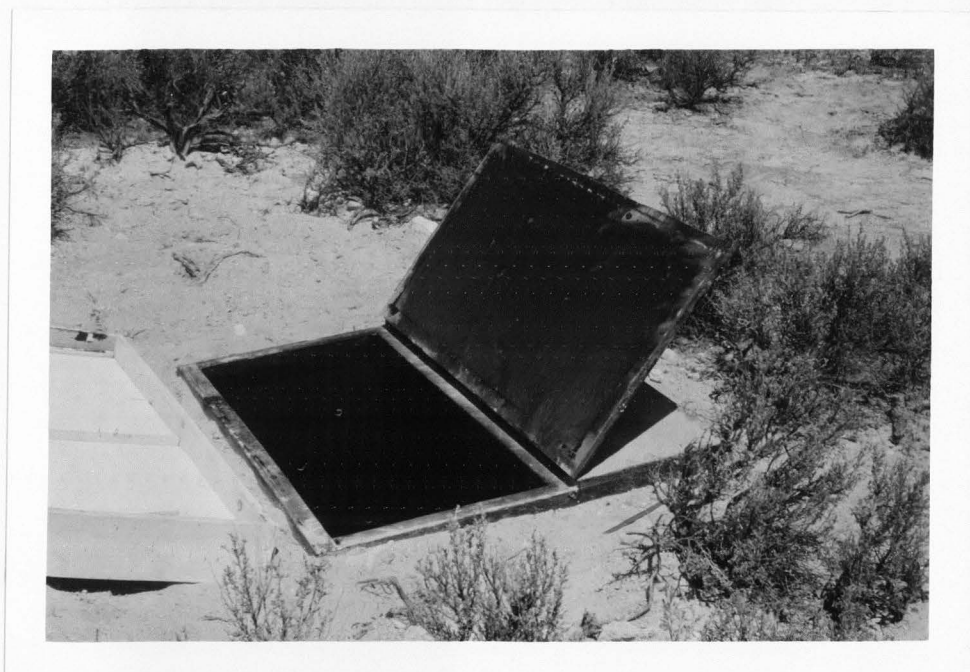
Figure 7. View of the root observation chamber open for root growth recording.
