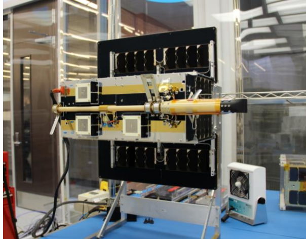
Figure 7: Stowed VDES Antenna aboard NORSAT-2 (Flight)
