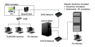
Figure 11: AOCS operation training using static closed loop test equipment and operation system
