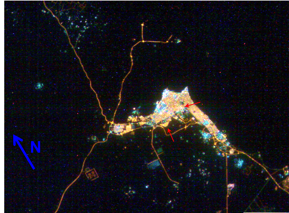
AeroCube-5 NFOV Camera (low altitude pass) ~ 90m GSD 18 May 2017 red arrows mark blue/green to yellow change
