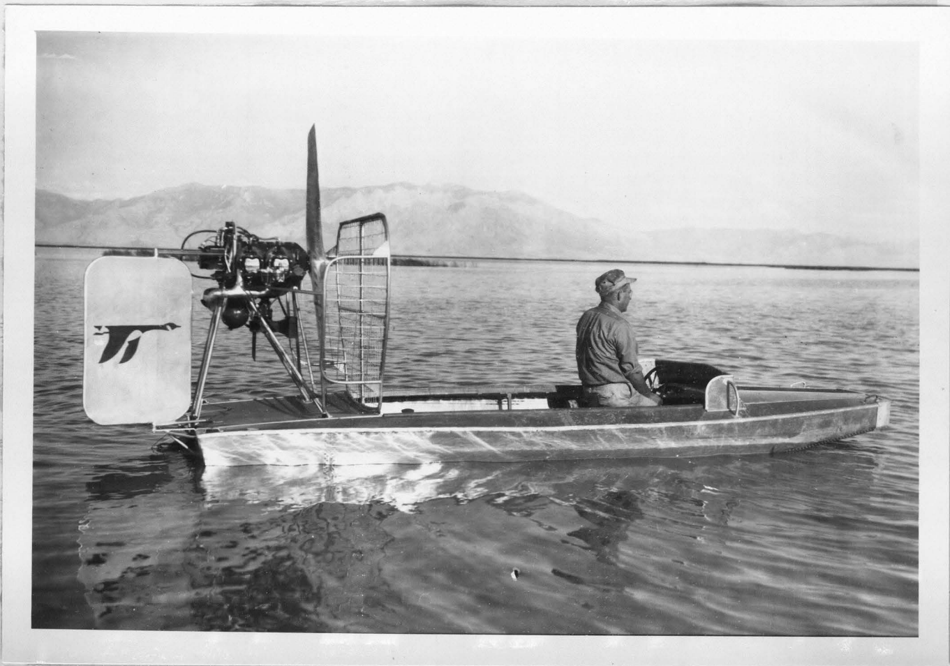
Figure 4. Air-thrust boat used in picking up waterfowl for examination. It can maneuver in shallow water and is easily transported. (Fish and Wildlife Service photo)
