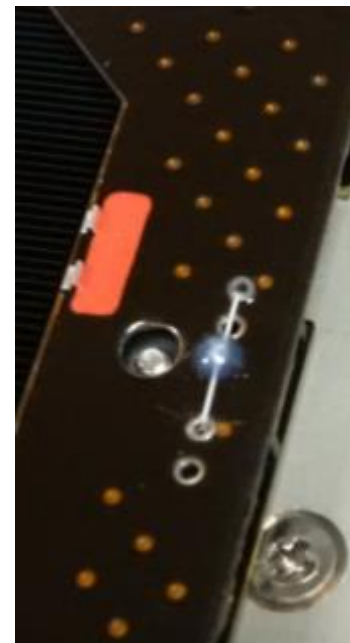
Intact tie-down after vibration testing
