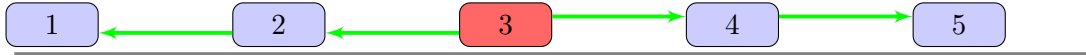
Fig. 3.6: Interaction of a 5-Member Platoon with Attacker at Position 3 with Adjacency Adjusted.
