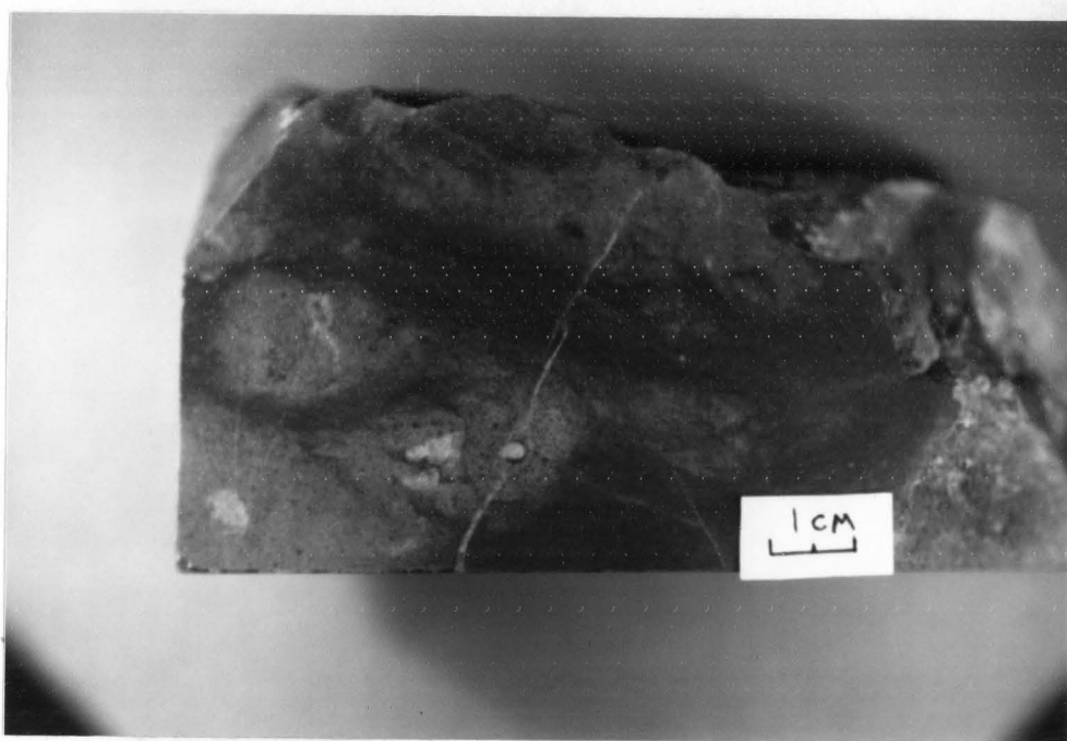
FIG. 28 - Photograph showing early dolomitized burrows with compaction features around them.
