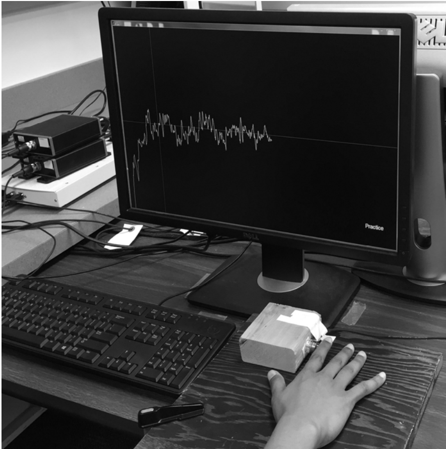
Figure 3-2. Study 1: Visual-motor tracking task apparatus and display. The horizontal line is the target line. The white line is the participant's produced force.
