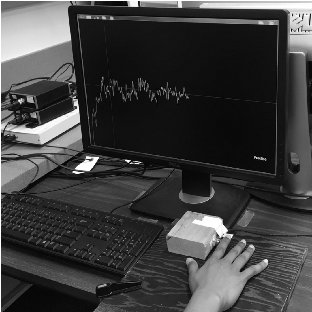
Figure 4-2. Study 2: Visual-motor tracking task apparatus and display. The horizontal line is the target line. The white line is the participant's produced force.
