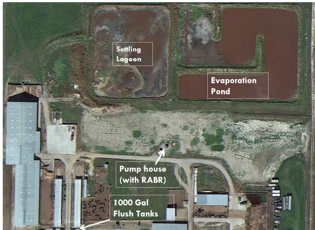
Fig. 7 Caine Dairy overhead photo. Waste management system is highlighted within the figure, including RABR setup at pumphouse.
