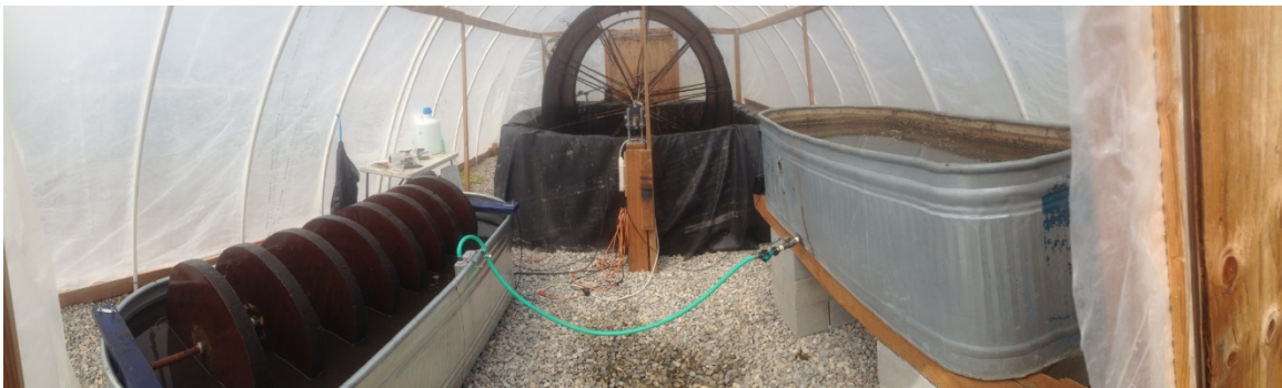
Fig. 8 Layout of RABR station at Caine Dairy. Left – Disc style RABR (200 gal, continuous flow) with 8 polystyrene discs of 2-foot diameter Back – Pilot Scale 6-foot diameter RABR (batch mode) Right – Reservoir for continuous flow disc reactor.
