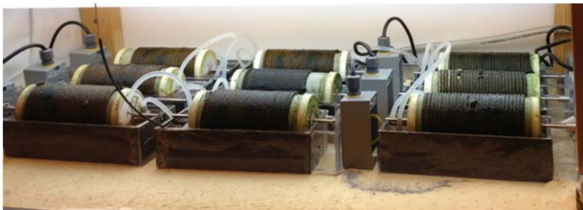
Fig. 3 RABR experimental setup. RABRs with This photograph depicts the algal biofilm on the RABRs 9 days after initial inoculation. Areal footprint of each individual reactor was measured to be 0.0338 \text{ m}^2 and total rope surface area was calculated to be 0.0305 \text{ m}^2 .
