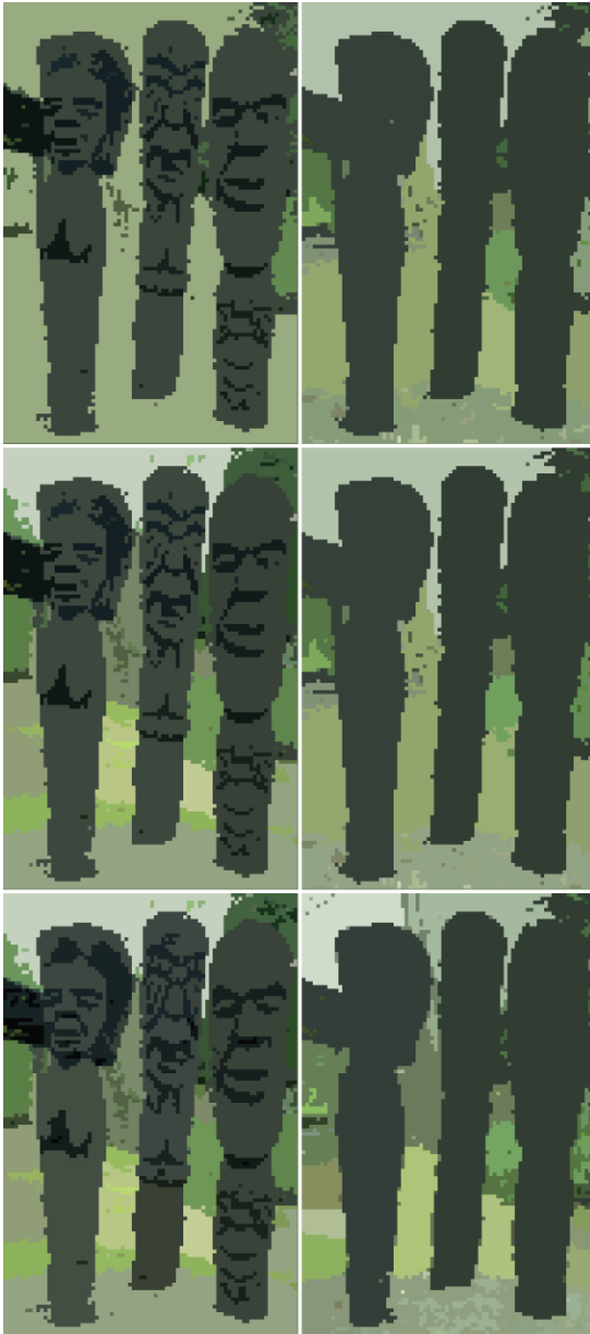
Figure 4.3: The comparison of the outputs of the SIMPLicity- RGB segmentation algorithm (shown on the left-hand side) and the outputs of the De-Texturing-LUV- SIMPLicity segmentation algorithm (shown on the right-hand side) for different values of k 's, where the top row presents the results for k = 3 , the middle row presents the results for k = 4 , and the bottom row presents the results for k = 5 .
