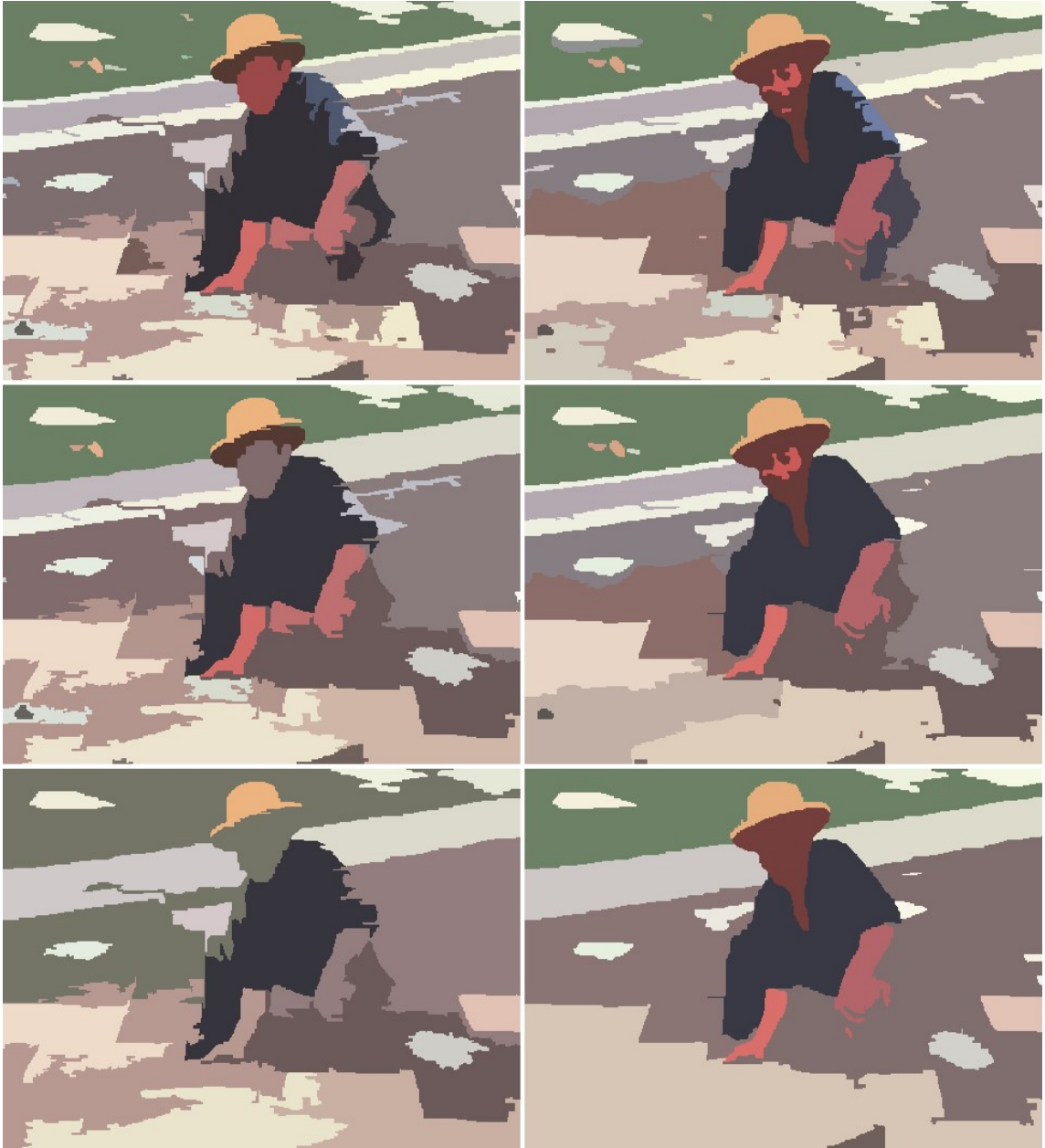
Figure 4.2: Comparison of the outputs of the SRM-RGB segmentation algorithm (shown on the left-hand side) and the outputs of the De-Texturing-YIQ-SRM segmentation algorithm (shown on the right-hand side) for different values of Q 's, where the top row presents the results for Q=4 , the middle row presents the results for Q=5 , and the bottom row presents the results for Q=6 .
