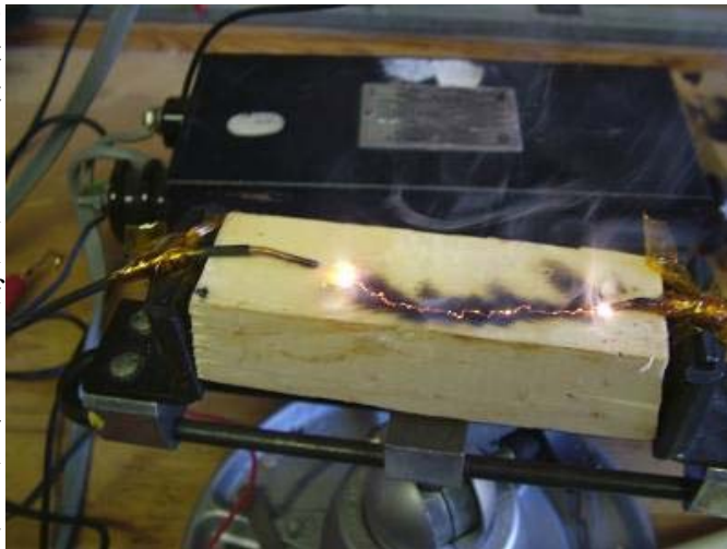
Figure 5: Conductive arc-track in wood
