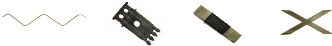
Figure 2 – Shear Connectors Tested, Left to Right: THiN Wall NU-Tie, HK Composite Tie, Thermomass CC and Thermomass X
