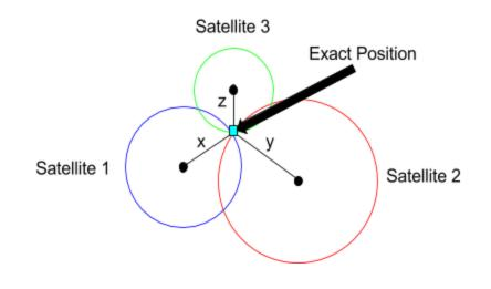
Imagining how this works three dimensionally isn't much different, however, now you are positioned on a sphere *x* distance from satellite 1, y distance from satellite 2, z distance from satellite 3, and a fourth satellite is required to account for the added dimension, w distance from satellite 4. (*Trilateration vs. Triangulation - How GPS Receivers Work*, gisgeography.com)
