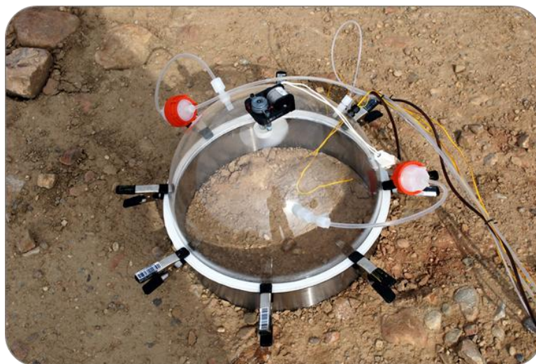
Figure 6. A picture of DFC, steel collar, and sampling equipment used to measure emissions.
