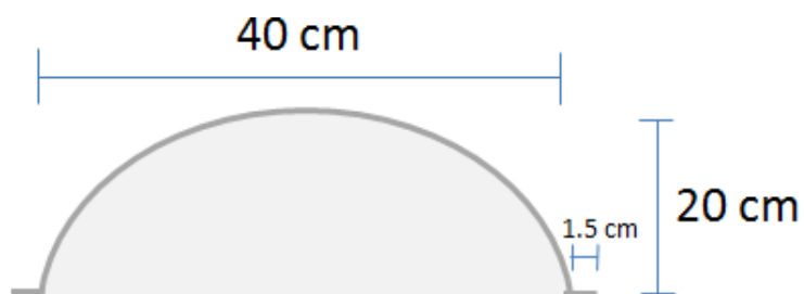
Figure 5. Cross-section of dynamic flux chamber dimensions.
