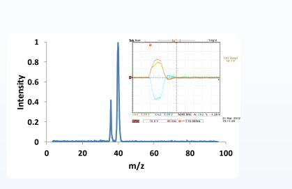
Improved BNG modulation (see inset) led to improved spectra. The above spectrum was collected using 122 eV Ar<sup>+</sup> ions. For the spectrum above, resolution is 25 at 10% peak height, and 40 at FWHM.
