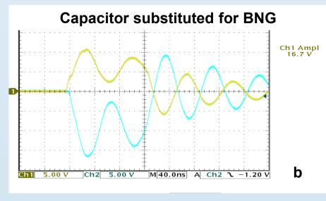
150  $\Omega$  resistors in series with both BNG
