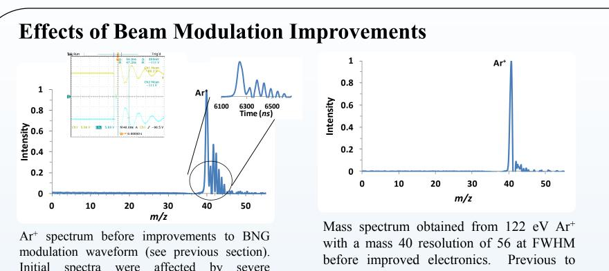
Initial spectra were affected by severe modulation defects, see insets.
