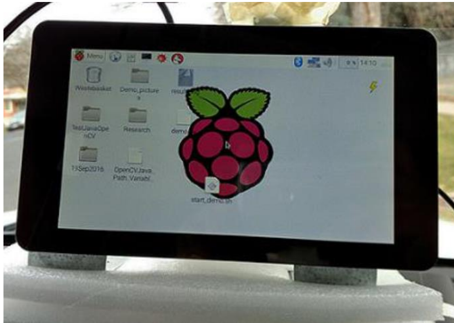
Fig. 4.1 Raspberry Pi Touchscreen Display: An RPi touchscreen display is attached to an RPi (behind it) and mounted next to the windshield of a Jeep Wrangler
