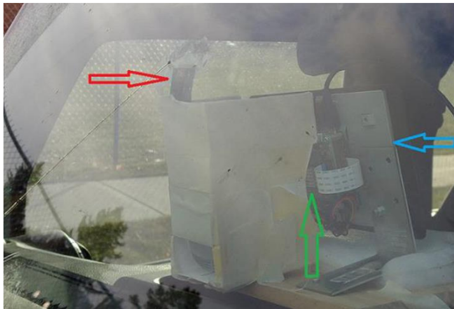
Fig. 4.2 Raspberry Pi Camera Board, and Raspberry Pi Computer Board: An RPi camera board v2 (red arrow) attached to small cardboard box for balance and taped to windshield; RPi computer (green arrow); RPi monitor (blue arrow)
