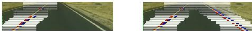
Fig. 4.10 Scanlines (white lines) and Spikes (red and blue lines) Used to Detect Lanes
