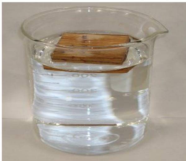
Fig. 3.5. A 48-hour soaking test.
