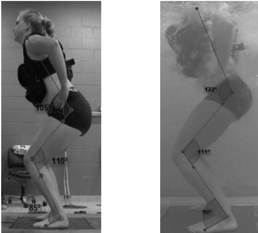
Figure 1. Example of angle measurements for data analysis of the land and aquatic landings using the digital goniometer tool from Kinovea. Smaller angles indicated increased joint flexion and larger angles indicated decreased joint flexion.
