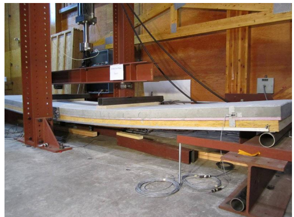
Figure 209, Wood-concrete composite floor undergoing testing. Equilibrium Consulting
