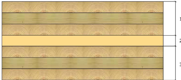
Figure 203, 3-ply CLT panel with mineral wool gap. CLT Handbook
