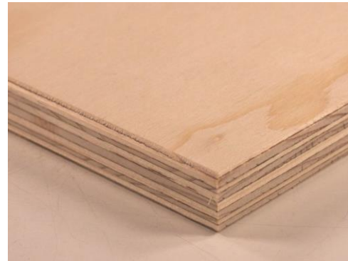
Figure 219, Plywood layer construction.
