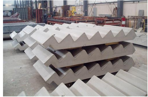
Figure 242, Precast concrete stair runs.
