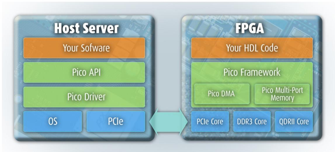
Figure 5.1: The vendor implemented Pico framework software stack gives easy to use APIs to tweak hardware design parameters on the FPGA logic. The stream framework may be used to interact directly with the HMC. Adopted from [15]
