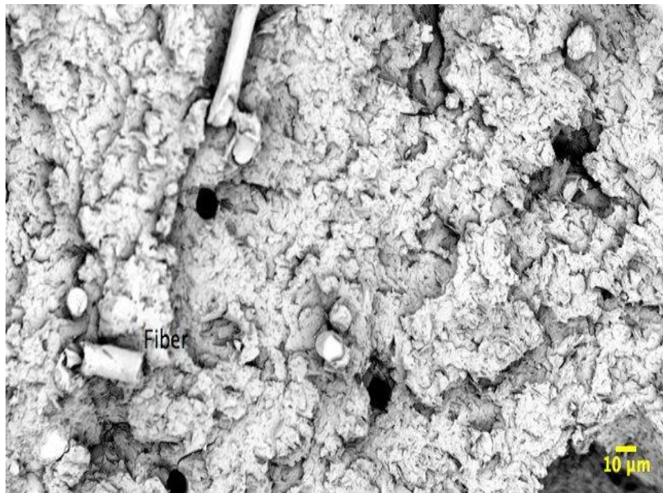
Figure 16 - SEM of 30/70 wt% GF/Nylon composites
