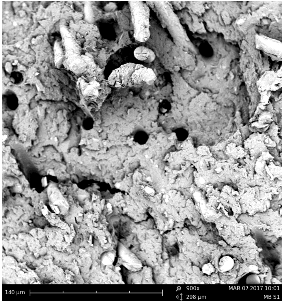
Figure 20 - SEM of 15/15/70 wt% 0621/GF/Nylon composites
