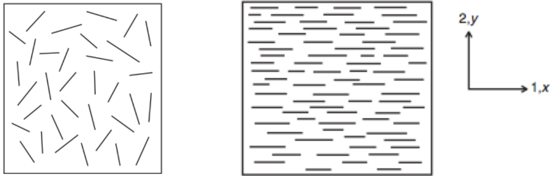
Figure 21 - Randomly oriented discontinuous fiber lamina (left) vs uniformly aligned discontinuous fiber lamina [Mallick]
