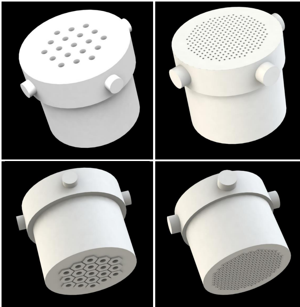
Figure 2-30. Upper plenum CAD models: reduced (19 assemblies, left) and full version (253 assemblies, right)
