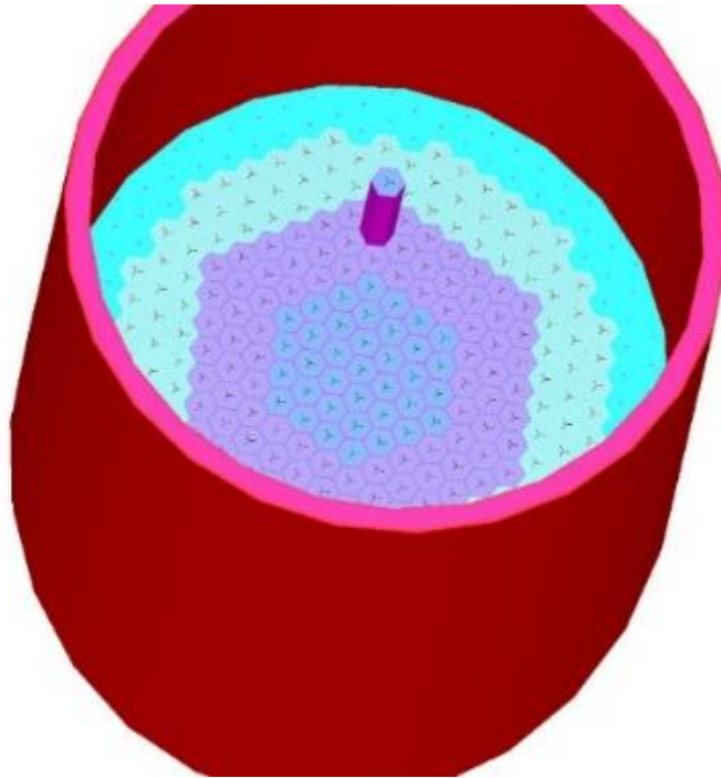
Figure 3-5. 3D view of the SCALE core model; assemblies are grouped in three radial rings and one assembly is partially extracted
