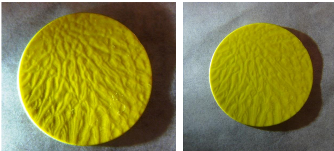
Figure 112: Striations on Matrimid phase separated films after casting them with VTMS in casting solution.
