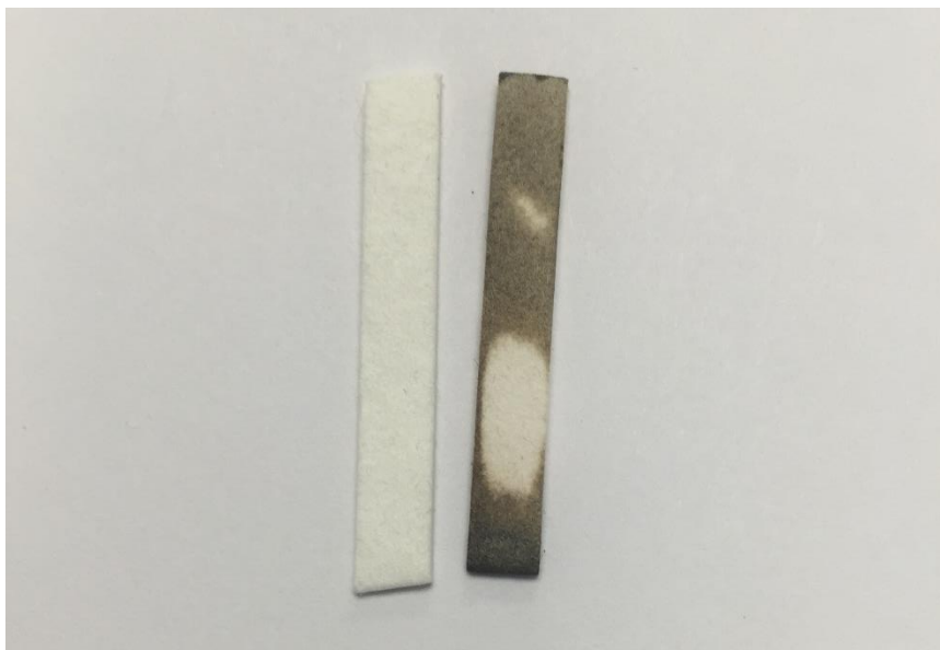
Figure 108: Lead acetate test for gas evolved from TPD from the unconditioned sample (left) and H 2 S conditioned sample (right). Both CMS samples were pyrolyzed at 550 °C with 15 ppm Cl 2 in Ar atmosphere.
