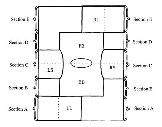
Figure 2. Layout of the Various Garment Parts in a Two Dimensional Fabric
