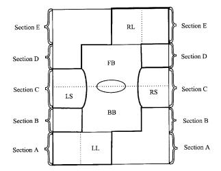
Layout of the Various Garment Parts in a Two Dimensional Fabric
