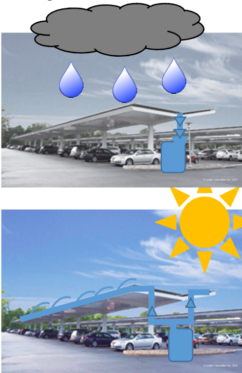
Figure 5. Our design will collect rainwater on rainy days and use it to cool and clean panels on hot sunny days.
