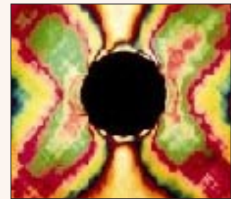
Fig. 6. Stress pattern on a composite (heterogeneous) material plate with a hole
