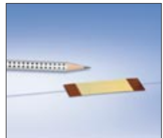
Top: A number of optical strain gauges (based on the Bragg grating) can be connected via a single glass fibre to a measuring instrument called an interrogator. Above: HBM's optical strain gauges are about 30 mm long.
