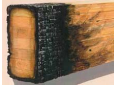
Char protects the inner core
