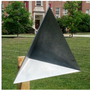
(b) Corner reflector, RCS = 596m^2 .
