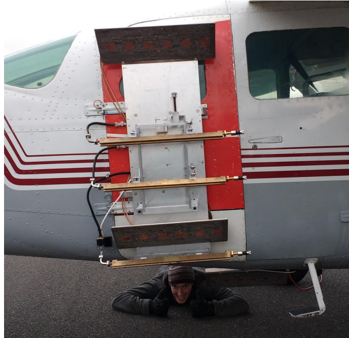
Figure 5.2: Antennas installation on the airplane. The top antenna is the first S-band receiver. The next two are the two Ka-band receive antennas. Next, the second S-band receive antenna. The Ka-band transmit antenna is mounted at the bottom. The S-band transmit antenna is mounted on the belly port of the airplane.
