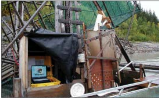
This video system continuously records fish passing through the fishwheel and captures the information on a laptop for later analysis.
