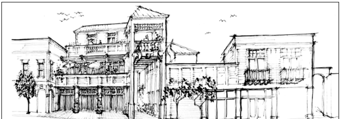
Figure 7.5: Illustrative sketches Main Street: variations in height, setbacks, and rooftop shapes create distinct building definition. Windows, balconies, and entrances facing the street promote transparency and are visually appealing. (Source: San Mateo County AIA, Half Moon Bay Charrette 1990)
