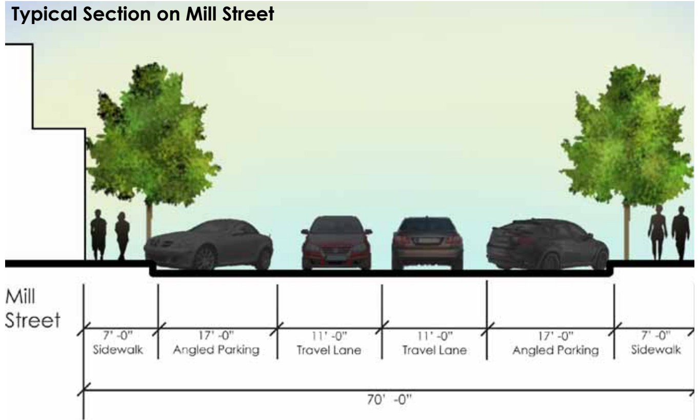
Figure 4.14: Typical Section on Mill Street
