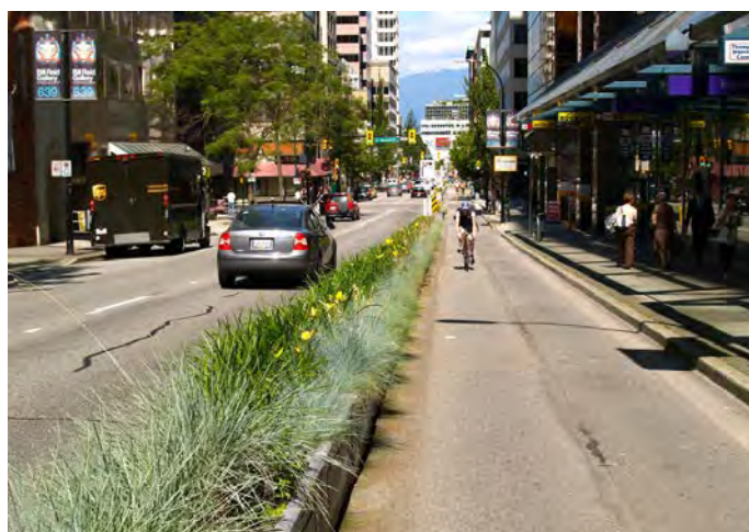
Figure 2.1: An Example of incorporating vegetation and grade separation between bikes and vehicles.
