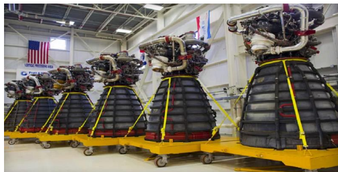
Figure 1. Space shuttle main engines (RS-25) manufactured by Aerojet Rocketdyne containing superalloy components joined with advanced braze alloys. 3
