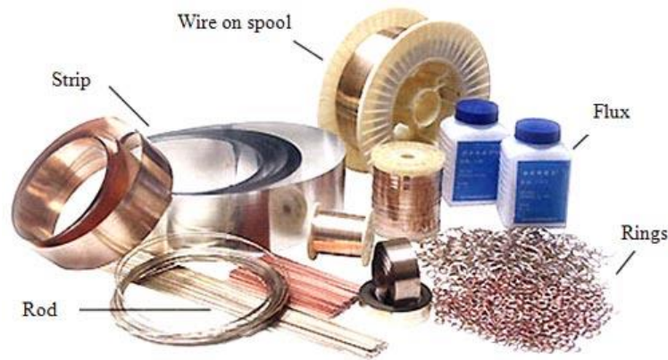
Figure 8. Various solid forms of braze alloys used in industry. 18
