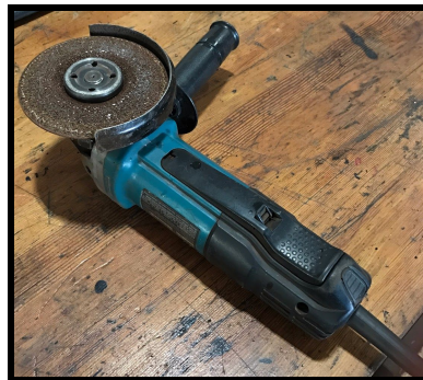
Figure 40. The angle grinder used to remove the oil coating on the material for the column.
