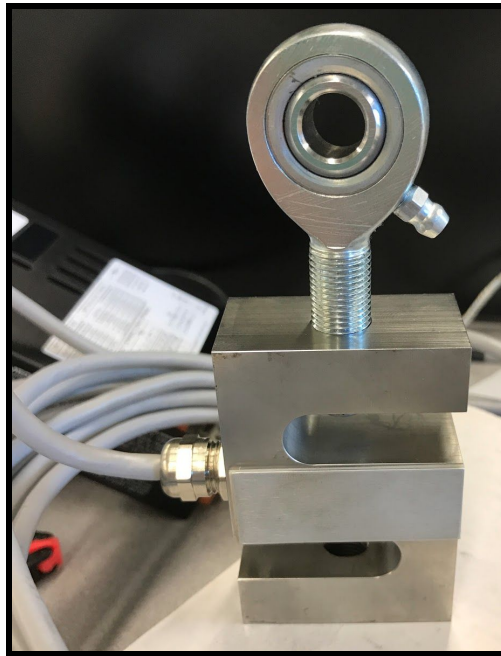
Figure 71. An image of the load cell connected to the rod end.
