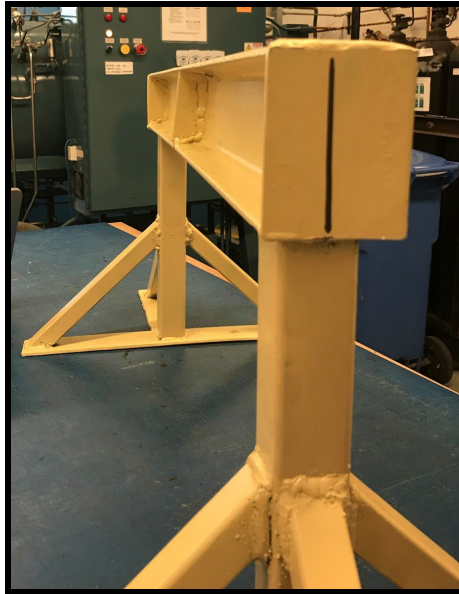
Figure 77. An image of the sawhorse after testing was completed. It is obvious from this picture that the structure yielded at the gusset.
