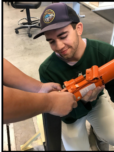
Figure 74. An image of the ram being connected to the attachment plate.
