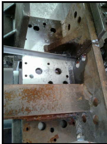
Figure 51. An image of the pre-welded structure after a portion of it was removed on the horizontal bandsaw.
