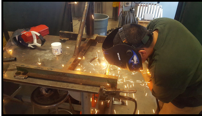
Figure 53. An image of Octavio welding the strong floor plates to the bottom of the engine stand.
