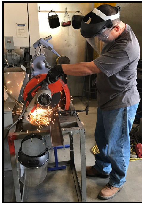
Figure 47. An image of Octavio attempting to cut the I-beam using a chop saw.
