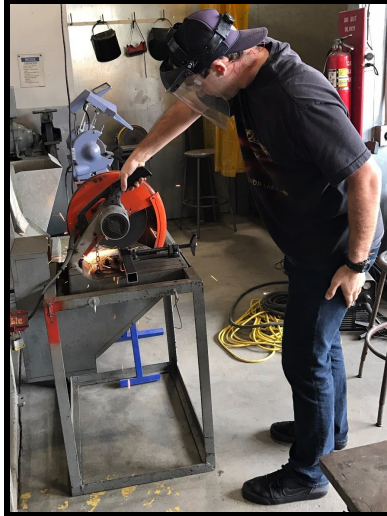
Figure 41. An image of Austin cutting the material for the column to size, using a chop saw.
