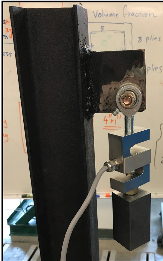
Figure 73. An image of the rod end, load cell, and load cell coupler attached to the ram connection plate.
