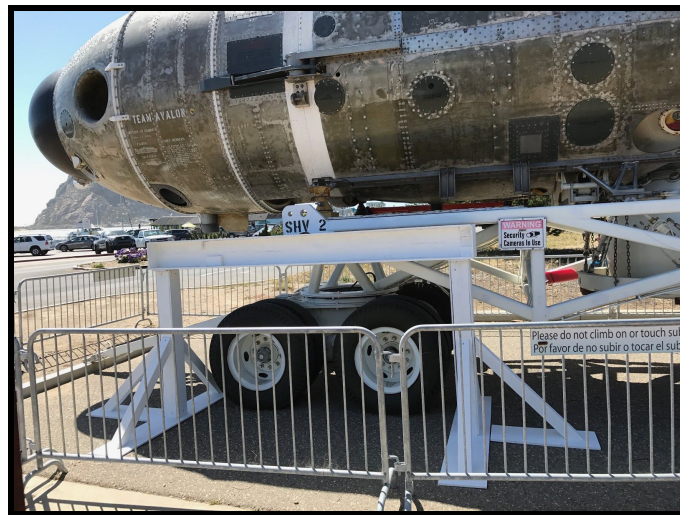
Figure 80. An image of the sawhorse placed up against the trailer. This is where the sawhorse will actually sit upon installation.
