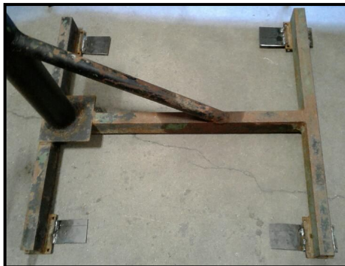
Figure 54. An image of the four strong floor plates after they were welded to the base of the engine stand.
