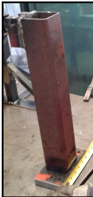
Figure 48. An image of the moment column before it was welded to the fixture base plate.
