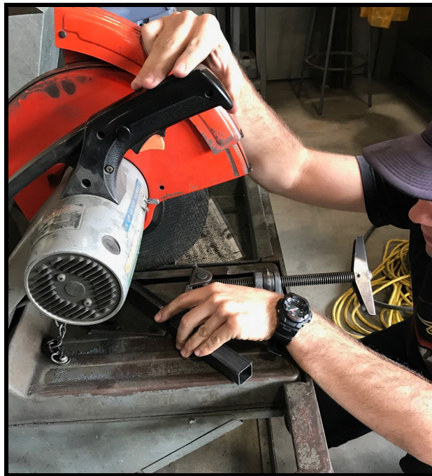
Figure 43. An image of Austin setting up the chop saw in preparation for making the miter cuts on the struts.
