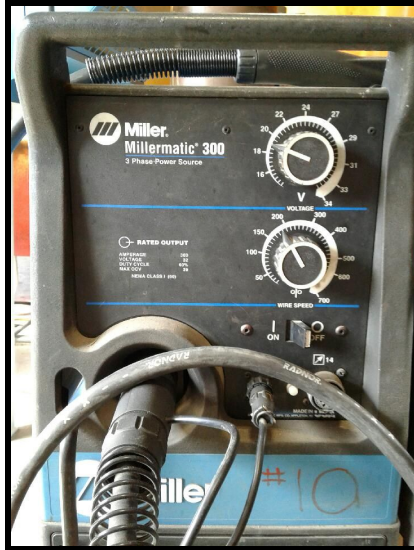
Figure 44. An image of the Miller MIG welder used for all welding operations.
