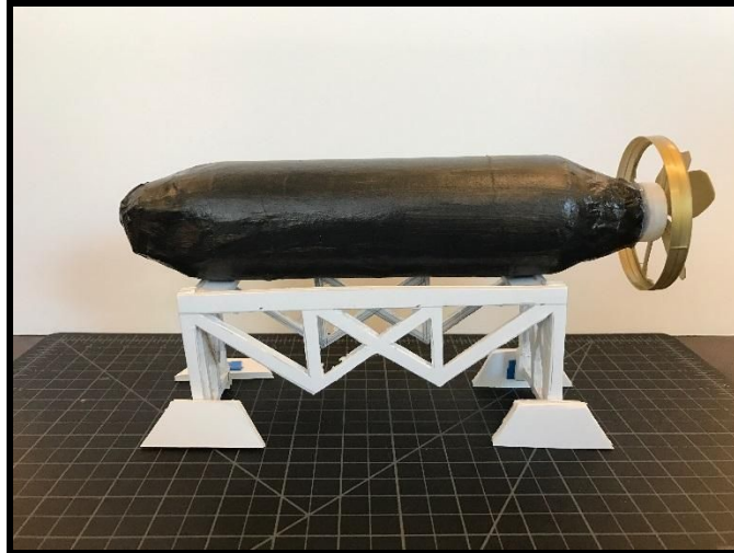
Figure 14. A concept model of the DSRV, the trailer it currently sits on, and Potential Solution #3. Note that the bolting mechanisms have been left off for the sake of simplicity in the model.
