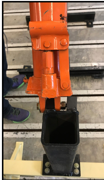
Figure 68. An image highlighting the induced eccentricity in the load case due to the hydraulic ram not working upside down.
