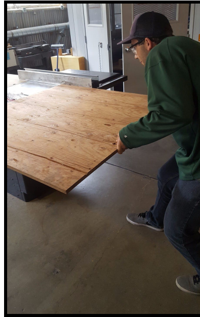
Figure 58. An image of the back plate being cut on the table saw.
