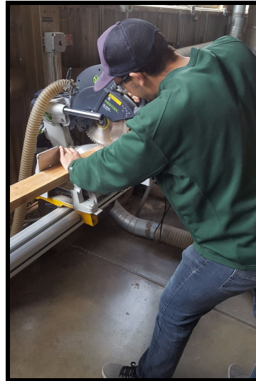
Figure 61. An image of the miter cuts being performed on the compound miter saw.
