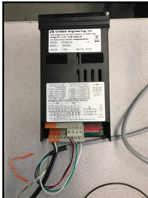
Figure 70. An image of the load cell connected to the load cell indicator.
