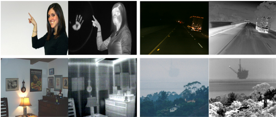
Figure 2: Visible vs. Infrared camera
