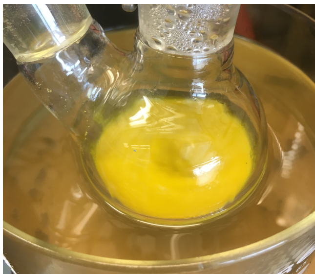
Figure 2. Synthesis occurring in round bottom flask dipped into an oil bath maintained at 65 °C.
