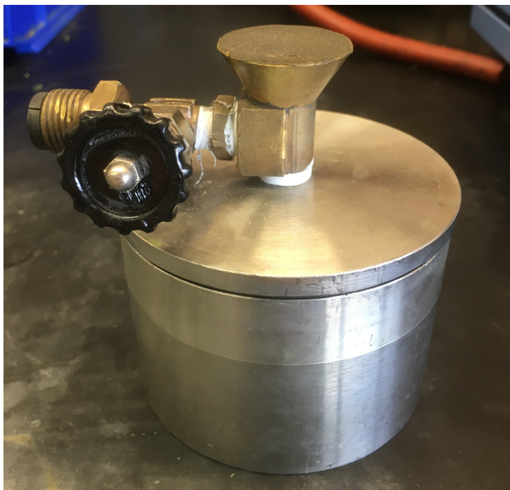
Figure 3. Vessel containing synthesis reactants and balls for ball milling procedure.
